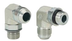
HY-TECH hydraulic fluid adapter, elbow, plated steel body, (1) -10 male JIC 37 deg and (1) -8 male o-ring boss. Package of 2.
