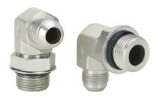
HY-TECH hydraulic fluid adapter, elbow, plated steel body, (1) -10 male JIC 37 deg and (1) -12 male o-ring boss. Package of 2.
