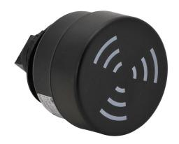
WERMA audible alarm buzzer, 80 dB at 1m, 2.1 kHz tone frequency, pulse tone(s), 115 VAC/VDC, 22mm, panel mount, ABS/polycarbonate housing, black, IP65.
