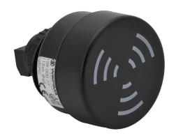
WERMA audible alarm buzzer, 80 dB at 1m, 2.1 kHz tone frequency, continuous tone(s), 115 VAC/VDC, 22mm, panel mount, ABS/polycarbonate housing, black, IP65.
