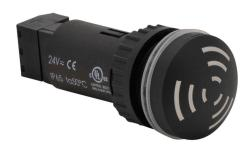
WERMA audible alarm buzzer, 80 dB at 10cm, 2.4 kHz tone frequency, pulse tone(s), 24 VAC/VDC, 22mm, panel mount, glass fiber reinforced polyamide housing, black, IP65.
