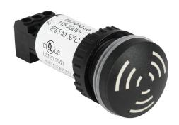
WERMA audible alarm buzzer, 80 dB at 10cm, 2.4 kHz tone frequency, pulse tone(s), 115-230 VAC, 22mm, panel mount, glass fiber reinforced polyamide housing, black, IP65.
