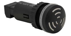
WERMA audible alarm buzzer, 80 dB at 10cm, 2.4 kHz tone frequency, continuous tone(s), 115 VAC/VDC, 22mm, panel mount, glass fiber reinforced polyamide housing, black, IP65.
