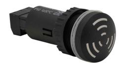
WERMA audible alarm buzzer, 80 dB at 10cm, 2.4 kHz tone frequency, continuous tone(s), 115 VAC/VDC, 22mm, panel mount, glass fiber reinforced polyamide housing, black, IP65.
