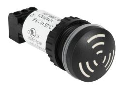
WERMA audible alarm buzzer, 80 dB at 10cm, 2.4 kHz tone frequency, continuous tone(s), 12/24 VAC/VDC, 22mm, panel mount, glass fiber reinforced polyamide housing, black, IP65.
