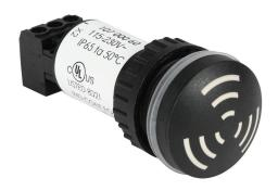
WERMA audible alarm buzzer, 80 dB at 10cm, 2.4 kHz tone frequency, continuous tone(s), 115-230 VAC, 22mm, panel mount, glass fiber reinforced polyamide housing, black, IP65.
