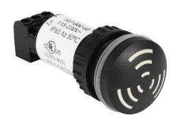
WERMA audible alarm buzzer, 80 dB at 10cm, 2.4 kHz tone frequency, continuous tone(s), 115-230 VAC, 22mm, panel mount, glass fiber reinforced polyamide housing, black, IP65.
