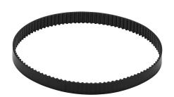
SureMotion timing belt, 0.08in MXL pitch, 1/4in wide, 106 tooth, 8.5in pitch length (circumference), polyurethane, polyester reinforced. Package of 3.
