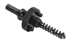
RUKO arbor assembly, type A2, 5/8-18 UNF, 7/16in hex shank. For use with 1-1/4 to 8-1/4in diameter bi-metal hole saws. Type A2 arbor, HSS 1/4in pilot bit, hex key and ejector spring included.
