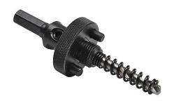
RUKO arbor assembly, type A2, 5/8-18 UNF, 7/16in hex shank. For use with 1-1/4 to 8-1/4in diameter bi-metal hole saws. Type A2 arbor, HSS 1/4in pilot bit, hex key and ejector spring included.
