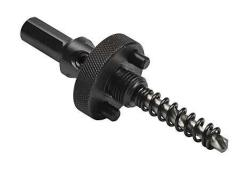
RUKO arbor assembly, type A5, 1/2-20 UNF, 3/8in hex shank. For use with 9/16 to 1-3/16in diameter bi-metal hole saws. Type A5 arbor, HSS 1/4in pilot bit, hex key and ejector spring included.
