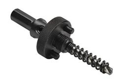
RUKO arbor assembly, type A5, 1/2-20 UNF, 3/8in hex shank. For use with 9/16 to 1-3/16in diameter bi-metal hole saws. Type A5 arbor, HSS 1/4in pilot bit, hex key and ejector spring included.
