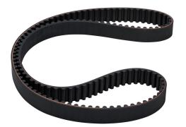
SureMotion timing belt, 8mm 8M pitch, 20mm wide, 130 tooth, 1040mm pitch length (circumference), neoprene, fiberglass reinforced.
