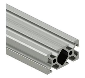
SureFrame 10 Series standard T-slotted rail, silver, 6063-T6 anodized aluminum alloy, cut to length, 1 x 2in profile, slot size 6.
