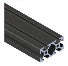
SureFrame 10 Series standard T-slotted rail, black, 6063-T6 anodized aluminum alloy, cut to length, 1 x 2in profile, slot size 6.
