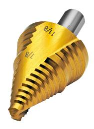
RUKO step drill bit, 2 steps, 7/8in and 1-1/8in, split point, high-speed steel (HSS), Titanium-Nitride (TiN) coated finish, 3/8in diameter 3-surface shank.
