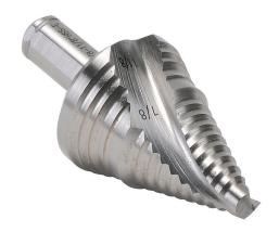
RUKO step drill bit, 2 steps, 7/8in and 1-1/8in, split point, 5% cobalt high-speed steel (HSSE-Co5), bright finish, 3/8in diameter 3-surface shank.
