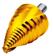
RUKO step drill bit, 5 steps, 7/8in, 1-1/8in, 1-7/32in, 1-1/4in and 1-3/8in, split point, high-speed steel (HSS), Titanium-Nitride (TiN) coated finish, 3/8in diameter 3-surface shank.
