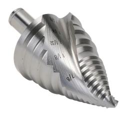
RUKO step drill bit, 5 steps, 7/8in, 1-1/8in, 1-7/32in, 1-1/4in and 1-3/8in, split point, 5% cobalt high-speed steel (HSSE-Co5), bright finish, 3/8in diameter 3-surface shank.
