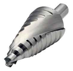
RUKO step drill bit, 9 steps, 13/32in, 9/16in, 5/8in, 11/16in, 3/4in, 13/16in, 7/8in, 15/16in and 1in, split point, high-speed steel (HSS), bright finish, 3/8in diameter 3-surface shank.
