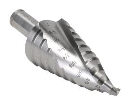
RUKO step drill bit, 9 steps, 13/32in, 9/16in, 5/8in, 11/16in, 3/4in, 13/16in, 7/8in, 15/16in and 1in, split point, 5% cobalt high-speed steel (HSSE-Co5), bright finish, 3/8in diameter 3-surface shank.
