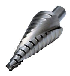
RUKO step drill bit, 12 steps, 3/16in, 1/4in, 5/16in, 3/8in, 7/16in, 1/2in, 9/16in, 5/8in, 11/16in, 3/4in, 13/16in and 7/8in, split point, high-speed steel (HSS), bright finish, 3/8in diameter 3-surface shank.
