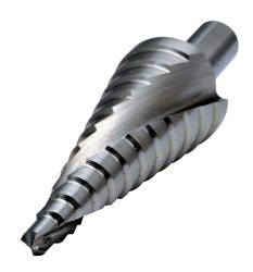
RUKO step drill bit, 12 steps, 3/16in, 1/4in, 5/16in, 3/8in, 7/16in, 1/2in, 9/16in, 5/8in, 11/16in, 3/4in, 13/16in and 7/8in, split point, high-speed steel (HSS), bright finish, 3/8in diameter 3-surface shank.
