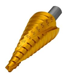
RUKO step drill bit, 12 steps, 3/16in, 1/4in, 5/16in, 3/8in, 7/16in, 1/2in, 9/16in, 5/8in, 11/16in, 3/4in, 13/16in and 7/8in, split point, high-speed steel (HSS), Titanium-Nitride (TiN) coated finish, 3/8in diameter 3-surface shank.
