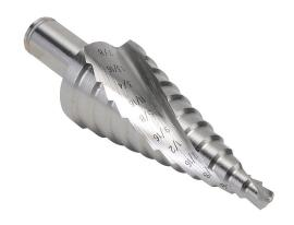
RUKO step drill bit, 12 steps, 3/16in, 1/4in, 5/16in, 3/8in, 7/16in, 1/2in, 9/16in, 5/8in, 11/16in, 3/4in, 13/16in and 7/8in, split point, 5% cobalt high-speed steel (HSSE-Co5), bright finish, 3/8in diameter 3-surface shank.
