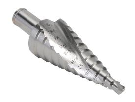
RUKO step drill bit, 12 steps, 3/16in, 1/4in, 5/16in, 3/8in, 7/16in, 1/2in, 9/16in, 5/8in, 11/16in, 3/4in, 13/16in and 7/8in, split point, 5% cobalt high-speed steel (HSSE-Co5), bright finish, 3/8in diameter 3-surface shank.
