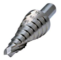
RUKO step drill bit, 9 steps, 1/4in, 5/16in, 3/8in, 7/16in, 1/2in, 9/16in, 5/8in, 11/16in and 3/4in, split point, high-speed steel (HSS), bright finish, 3/8in diameter 3-surface shank.
