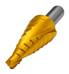
RUKO step drill bit, 9 steps, 1/4in, 5/16in, 3/8in, 7/16in, 1/2in, 9/16in, 5/8in, 11/16in and 3/4in, split point, high-speed steel (HSS), Titanium-Nitride (TiN) coated finish, 3/8in diameter 3-surface shank.
