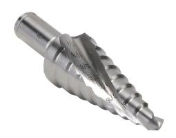
RUKO step drill bit, 9 steps, 1/4in, 5/16in, 3/8in, 7/16in, 1/2in, 9/16in, 5/8in, 11/16in and 3/4in, split point, 5% cobalt high-speed steel (HSSE-Co5), bright finish, 3/8in diameter 3-surface shank.
