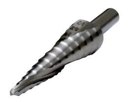
RUKO step drill bit, 13 steps, 1/8in, 5/32in, 3/16in, 7/32in, 1/4in, 9/32in, 5/16in, 11/32in, 3/8in, 13/32in, 7/16in, 15/32in and 1/2in, split point, high-speed steel (HSS), bright finish, 1/4in diameter 3-surface shank.
