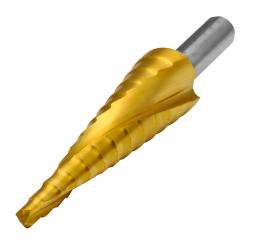
RUKO step drill bit, 13 steps, 1/8in, 5/32in, 3/16in, 7/32in, 1/4in, 9/32in, 5/16in, 11/32in, 3/8in, 13/32in, 7/16in, 15/32in and 1/2in, split point, high-speed steel (HSS), Titanium-Nitride (TiN) coated finish, 1/4in diameter 3-surface shank.
