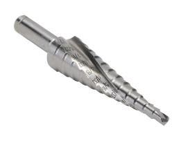
RUKO step drill bit, 13 steps, 1/8in, 5/32in, 3/16in, 7/32in, 1/4in, 9/32in, 5/16in, 11/32in, 3/8in, 13/32in, 7/16in, 15/32in and 1/2in, split point, 5% cobalt high-speed steel (HSSE-Co5), bright finish, 1/4in diameter 3-surface shank.
