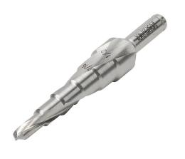
RUKO step drill bit, 6 steps, 3/16in, 1/4in, 5/16in, 3/8in, 7/16in and 1/2in, split point, high-speed steel (HSS), bright finish, 1/4in diameter 3-surface shank.
