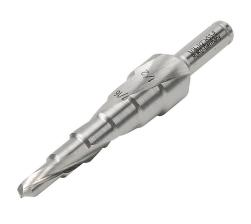
RUKO step drill bit, 6 steps, 3/16in, 1/4in, 5/16in, 3/8in, 7/16in and 1/2in, split point, high-speed steel (HSS), bright finish, 1/4in diameter 3-surface shank.
