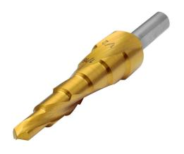
RUKO step drill bit, 6 steps, 3/16in, 1/4in, 5/16in, 3/8in, 7/16in and 1/2in, split point, high-speed steel (HSS), Titanium-Nitride (TiN) coated finish, 1/4in diameter 3-surface shank.
