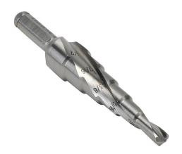
RUKO step drill bit, 6 steps, 3/16in, 1/4in, 5/16in, 3/8in, 7/16in and 1/2in, split point, 5% cobalt high-speed steel (HSSE-Co5), bright finish, 1/4in diameter 3-surface shank.
