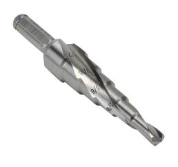
RUKO step drill bit, 6 steps, 3/16in, 1/4in, 5/16in, 3/8in, 7/16in and 1/2in, split point, 5% cobalt high-speed steel (HSSE-Co5), bright finish, 1/4in diameter 3-surface shank.
