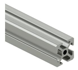
SureFrame 10 Series standard T-slotted rail, silver, 6063-T6 anodized aluminum alloy, cut to length, 1 x 1in profile, slot size 6.
