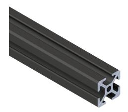
SureFrame 10 Series standard T-slotted rail, black, 6063-T6 anodized aluminum alloy, cut to length, 1 x 1in profile, slot size 6.
