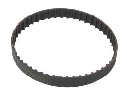
SureMotion timing belt, 1/5in XL pitch, 3/8in wide, 50 tooth, 10in pitch length (circumference), neoprene, fiberglass reinforced.
