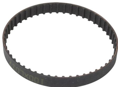
SureMotion timing belt, 1/5in XL pitch, 3/8in wide, 50 tooth, 10in pitch length (circumference), neoprene, fiberglass reinforced.
