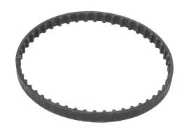
SureMotion timing belt, 1/5in XL pitch, 1/4in wide, 50 tooth, 10in pitch length (circumference), neoprene, fiberglass reinforced.
