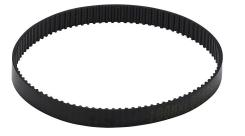
SureMotion timing belt, 0.08in MXL pitch, 1/4in wide, 100 tooth, 8in pitch length (circumference), polyurethane, polyester reinforced. Package of 3.
