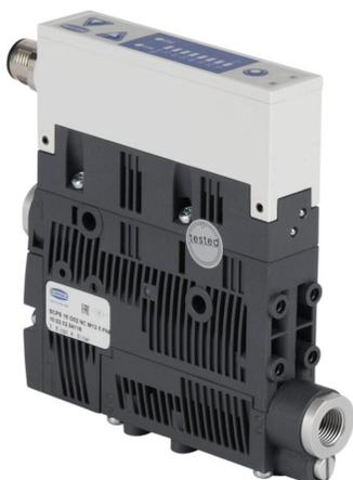
Schmalz compact vacuum ejector, 65.5 l/min (2.3 cfm) suction rate, G1/8 female BSPP inlet(s), G1/8 female BSPP vacuum port, air saving.
