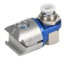
Schmalz PXT series suction cup mount, swivel, 5/16in (8mm) pushto-connect vacuum connection, G1/4 female BSPP cup connection, aluminum alloy. For use with D30-I profile.
