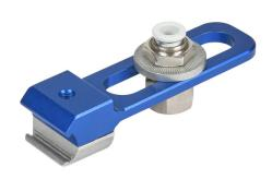
Schmalz PXT series suction cup mount, slotted, 5/16in (8mm) push-to-connect vacuum connection, G1/4 female BSPP cup connection, aluminum alloy. For use with D30-I profile.
