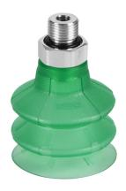
Schmalz vacuum suction cup, bellows, round, 2 fold(s), 30mm, Elastodur, G1/8 male BSPP.
