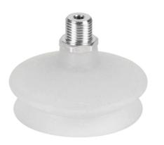
Schmalz vacuum suction cup, bellows, round, 1 fold(s), 63mm, silicone, G1/4 male BSPP.
