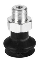
Schmalz vacuum suction cup, bellows, round, 1 fold(s), 20mm, nitrile rubber, G1/8 male BSPP.
