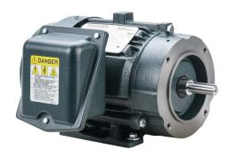
Toshiba SD premium efficiency AC induction motor, high-performance inverter duty and severe duty, 1/2hp, 3-phase, 230/460 VAC, 1200rpm, TEFC, NEMA 56C frame, cast iron, C-face/rigid base mount.
