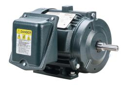
Toshiba SD premium efficiency AC induction motor, high-performance inverter duty and severe duty, 1/2hp, 3-phase, 230/460 VAC, 1200rpm, TEFC, NEMA 56 frame, cast iron, rigid base mount.
