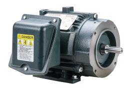
Toshiba SD premium efficiency AC induction motor, high-performance inverter duty and severe duty, 1/2hp, 3-phase, 230/460 VAC, 1800rpm, TENV, 56C frame, cast iron, C-face/rigid base mount.
