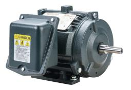
Toshiba SD premium efficiency AC induction motor, highperformance inverter duty and severe duty, 1/2hp, 3-phase, 230/460 VAC, 1800rpm, TENV, NEMA 56 frame, cast iron, rigid base mount.
