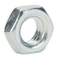
Metal Work rod nut, M8 x 1.25 thread, plated steel. For use with 20mm bore ISO 6432 cylinders.
