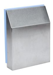
Stego hose-proof filter fan hood, fits  $4.88 \times 4.88$ in or  $4.92 \times 4.92$ in fan cutout, stainless steel, sanitary gasket, NEMA 4/4X, IP56, for increasing the protection classification of Stego Filter Fan and Filter Fan Plus fans and grilles.
